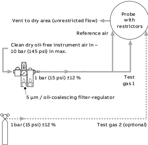
Fig. 6 AutoCal with air as test gas 1
