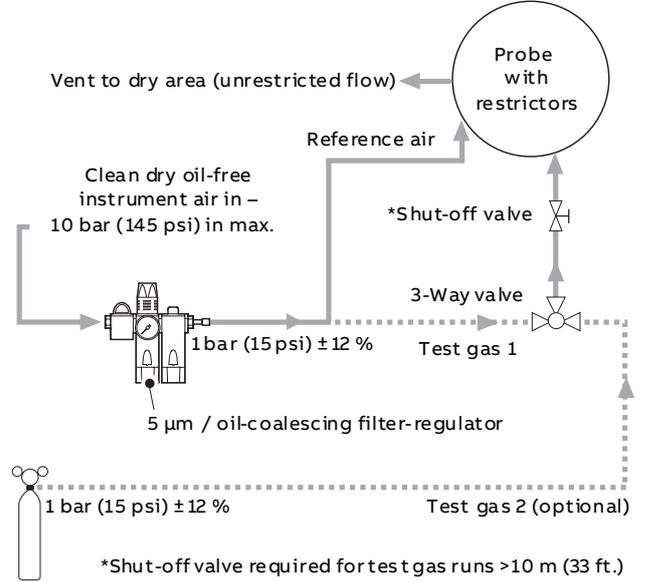
Fig. 8 Non-AutoCal with air as test gas 1
