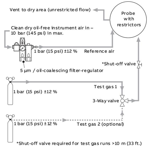
Fig. 9 Non-AutoCal with 2 test gases
