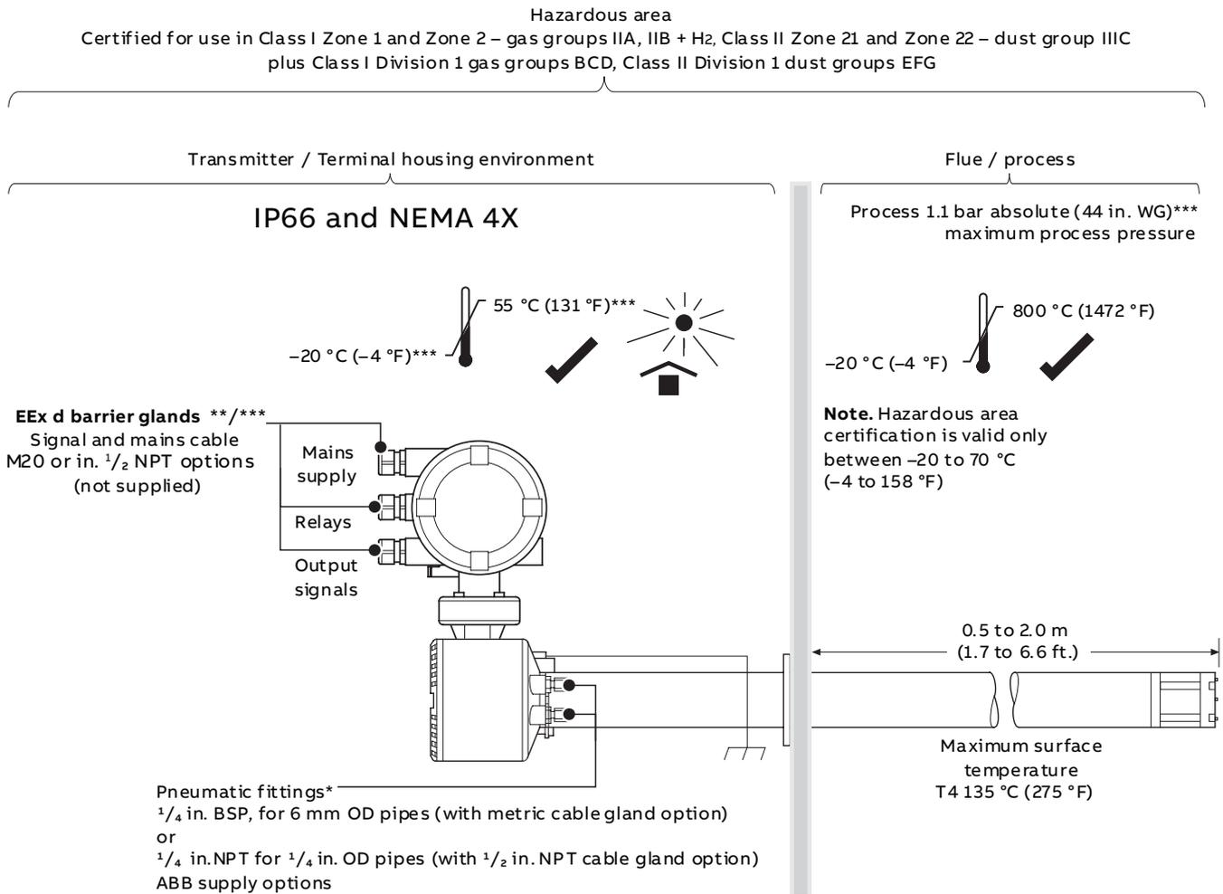
\*Transmitters do not contain a reference air supply for the probe. All external pneumatic fittings may be exchanged – they do not form part of the certified enclosure.
