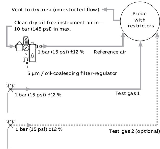
Fig. 7 AutoCal with 2 test gases
