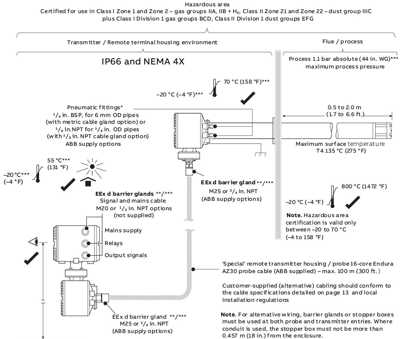
\*Transmitters do not contain a reference air supply for the probe. All external pneumatic fittings may be exchanged – they do not form part of the certified enclosure.
