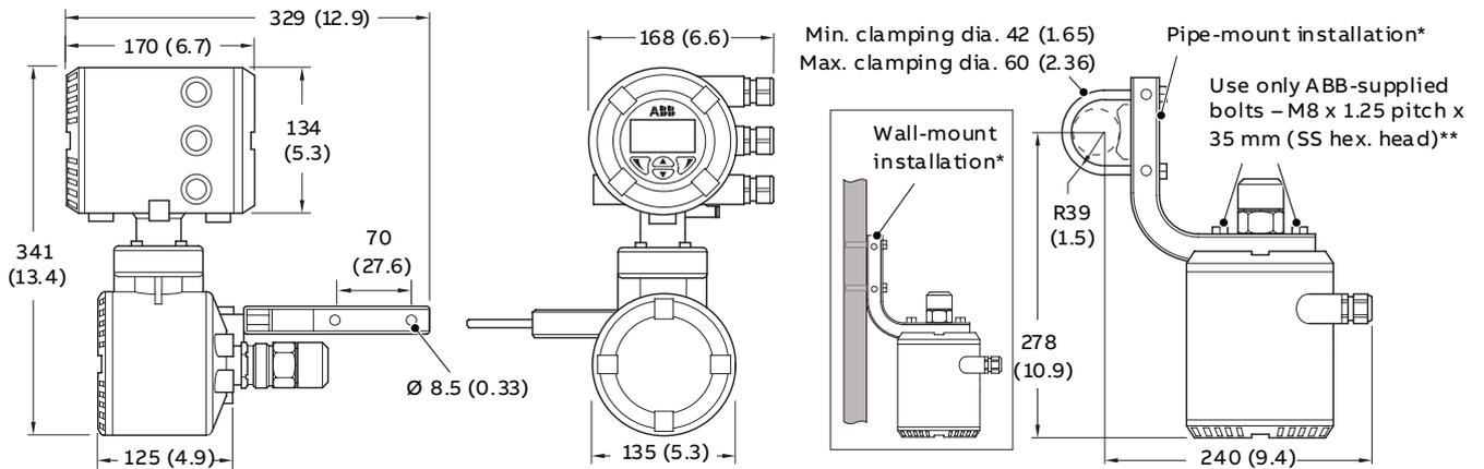
\*Wall- / Pipe-mount bracket plus U-bolt, pipe clamp and M8 fixings supplied as standard
