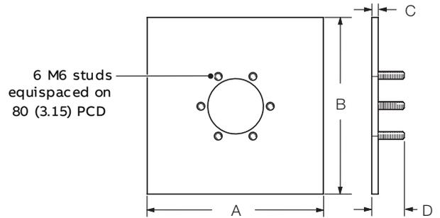
Standard mounting plate for 1.0 to 2 m (3.3 to 6.6 ft.) probes – Part No. AZ200 795
